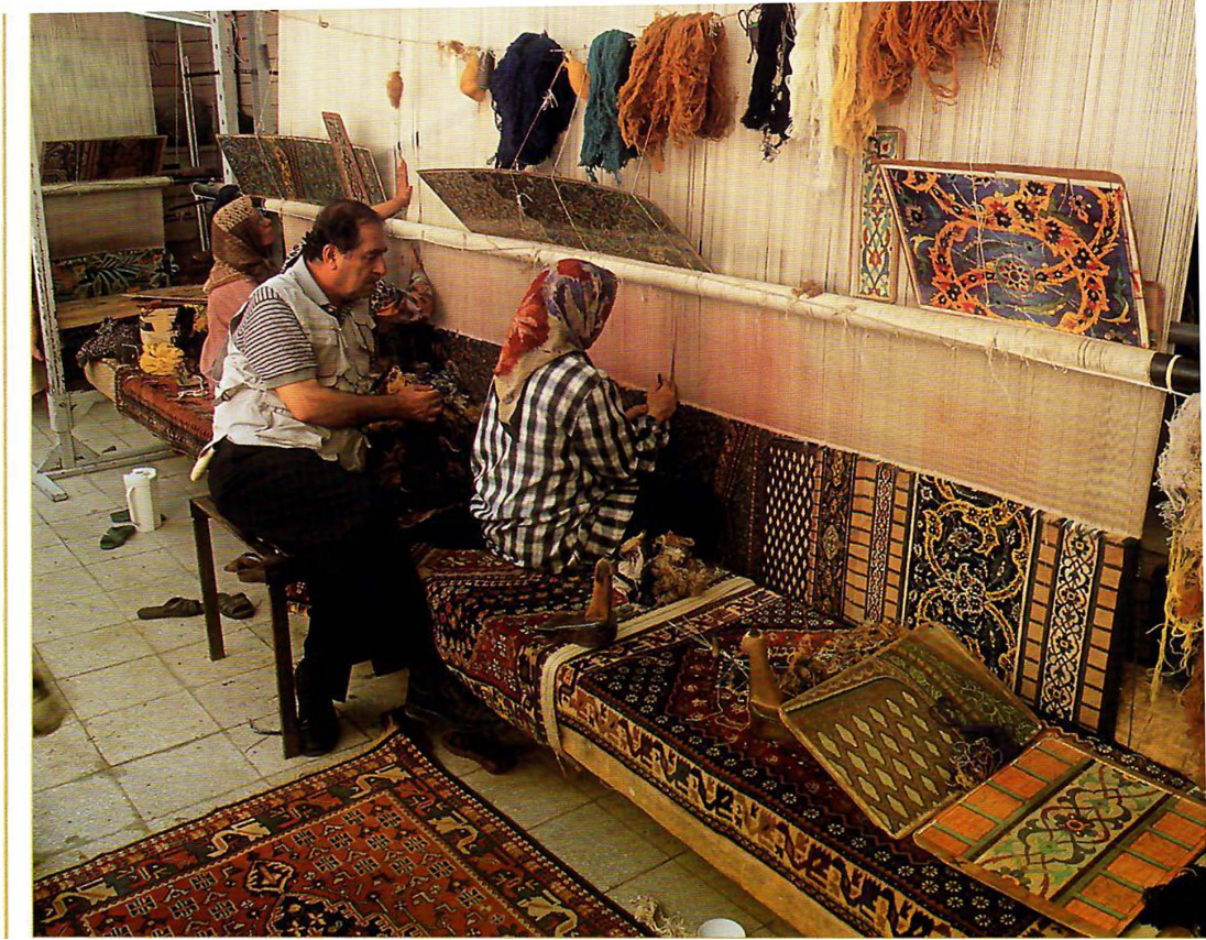
روی یک دار ثابت اصفهان weaving process on fixed loom in one of the carpet shop of Isfahan
